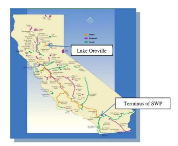
All of these water import systems cross seismic faults, and may be subject to interruption due to an earthquake. Those interruptions, however, may arise out of isolated breaks in the conveyance system, which may be repaired relatively quickly. The most vulnerable to a long-term outage
